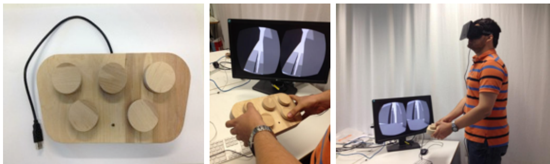
Figure 1: Self-developed, CNC-milled Controller (left); using controller and interacting with software (middle, right).
